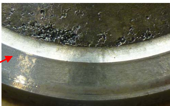
Corroded Intake Valve
